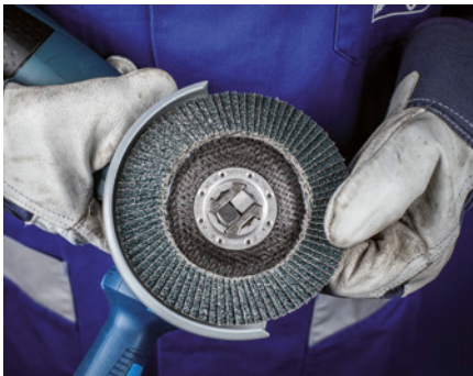
Place the tool on the X-LOCK quick-change system in a form-fitting manner.
