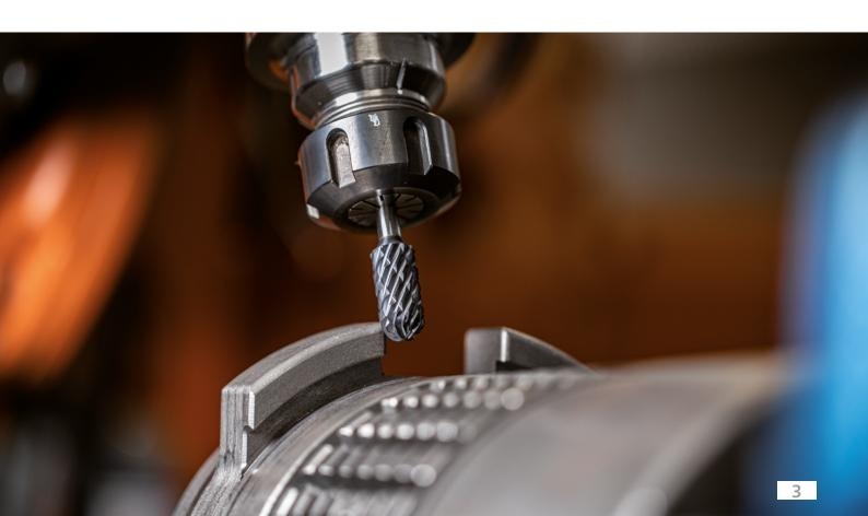
for use on steel and cast steel
