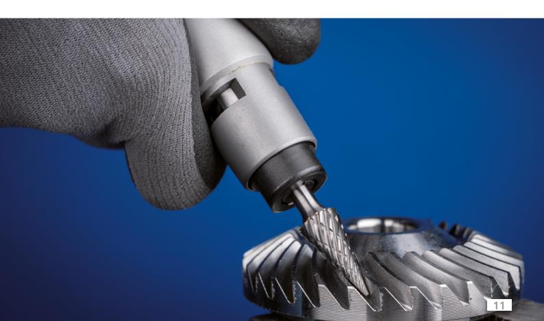
for use on steel and cast steel
