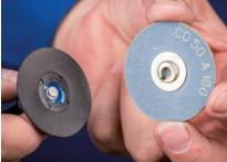
**Tool side:** Threaded connection with female thread (metal/plastic)
