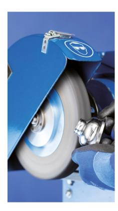
POLINOX non-woven tools PNK consist of spiral-shaped, non-woven abrasive which is wound around a core and foamed up. The foam supports the non-woven component and positively impacts its tool life and abrasive performance. This particular bond results in non-woven wheels with a very good surface finish, high stock removal rate and long tool life.
