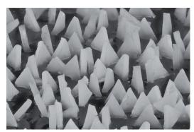
Of course most users value the enormous power of the triangular, precision-shaped high-performance abrasive. "**VICTO**GRAIN outperforms other, established solutions by up to 30% – with a consistently high degree of aggressiveness," said Heimann. It performs impressively in use. While other abrasives offer a similarly high level of aggressiveness at the beginning of use,
